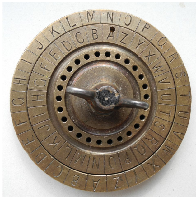
Figure 2. Cipher disc for substitution cipher, manufacturer: Linge, Pleidelsheim (Germany) (attribution: Hubert Berberich as public domain; source: https://commons.wikimedia.org/wiki/File:CipherDisk2000.jpg )
